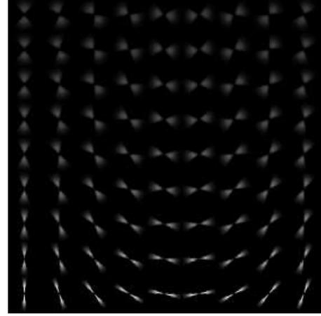
**Fig. 4.** Kernel topography: Oriented kernels for inference of continuity are bidirectional, and their energy dissipates as a function of distance. Initially, the energy is dispersed (top row), but becomes more focused (bottom row).
