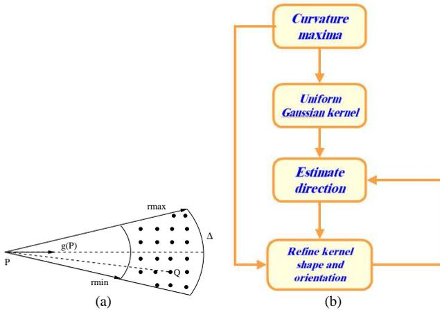
**Fig. 5.** (a) Redirection of the kernel in the next iteration; and (b) general flow of the algorithm.
